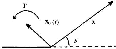
FIGURE 1. Vortex near a semi-infinite rigid plane.
